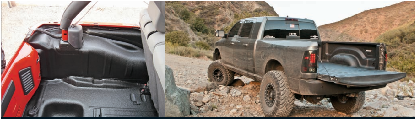
(Left) Count on spending 1.5 - 2 hours to complete a spray-on bed liner application. (Right) Bed liners come in a variety of applications that can include options such as UV and fade resistance and color matching.
