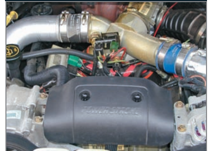
Late model 7.3L with the glow pug module. It is the silver box with the light green and black connectors.
