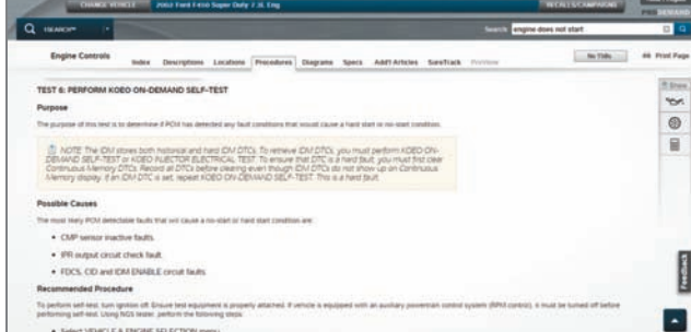
The scan tool test procedure for the 7.3L warning about performing the order correctly so that you do not erase codes before you ever see them.
