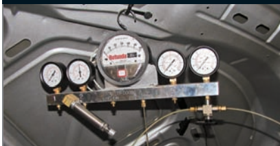
The correct way to connect a fuel pressure gauge on a 7.3L to check each head for fuel pressure. One gauge with a T handle to switch between heads. Spec is 45psi minimum, typical pressure is 60psi. If you see more than a 3psi difference in heads begin looking for a leak.
