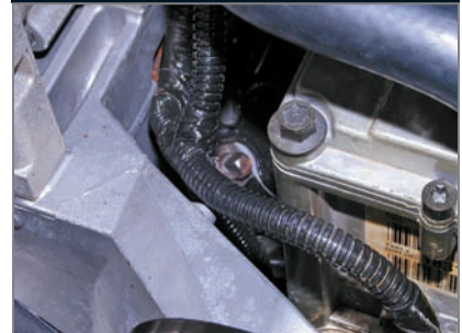
The quarter inch square head bolt is removed to access the fuel rail on the 7.3. Connect an adaptor and tube to your pressure gauge. This is the right head and is just behind and below the alternator bracket. Heads are the same on this engine so the port for the left head is at the back of the engine under the Intake and Turbo tubes.
