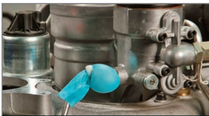
Performing the combustion gases in fuel system test on a 6.0L PSD.
