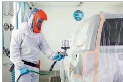
Hooded supplied-air respirators protect against dangerous chemicals, while offering comfort and a full field of vision.
