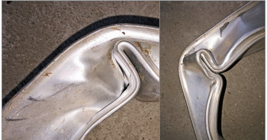
This is an extruded aluminum bumper reinforcement. In the severely kinked area you can see multiple indications of stress cracks and even fracturing of the material. Even at the bent area there are visible fractures.
