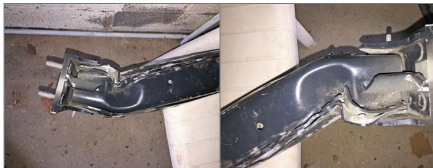
This is an aluminum uni-rail from a 2010 BMW. It is constructed of sheet aluminum with a cast front-mount bracket welded to it. You can see multiple deformities on the component, and in the "kinked" area where the metal has folded over itself you see stress cracking. The opposite side of the kinked area you can see a bend to the component. None of this damage is repairable.
