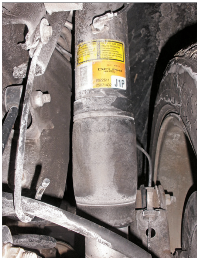
Electronically controlled versions of suspension dampers come in many forms, including air leveling shocks and struts.
