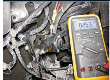
When diagnosing the Body Position Sensors, remove the linkage at one end and sweep with your voltmeter (key on) or scope just like you would a TPS looking for the classic potentiometer drop out. Min/Max should be used when a voltmeter is utilized to catch those intermittents.
