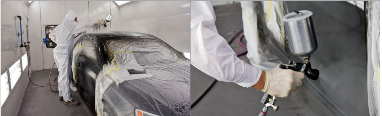
(Left) Avoid carrying contaminants into your booth by using only lint-free garments and cleaning your painting equipment. Pay attention to hoses since they can bring dirt into a booth if they're dragged against dirty shop floors. (Right) Always clean your paint guns with lint-free cloths before bringing them into your booth.
