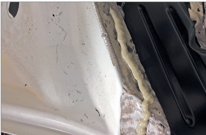
The adhesive is recommended for panel and weld bonding of aluminum roof and quarter panels, rear body and van side panels, and door skins.
