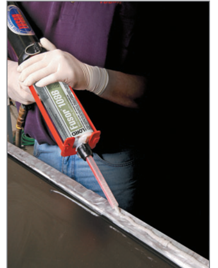
Ford has approved Fusor 108B /109B Metal Bonding Adhesive for repairing its aluminum-bodied F-150 pickup truck.
