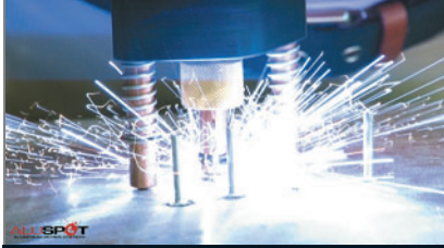
High speed photography and a specific power setting was used to capture this image for illustration purposes. It is best to eliminate excessive arc by lowering the power setting just enough so the pin welds have minimal spark to no spark.
