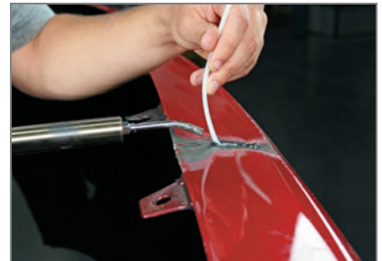
Use a thinner rod for the front of the bumper. Also, always try to keep the welder at a 45 degree angle.
