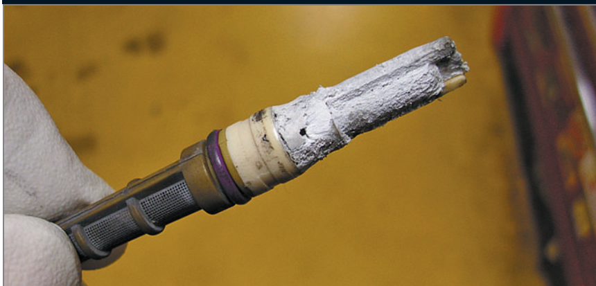
Sealant is a leading cause of compressor failures and system woes.
