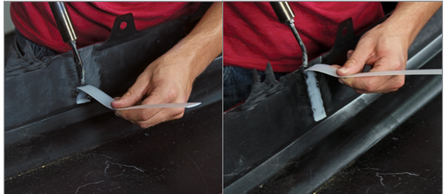
(Left) You'll use a wider welding rod on the back of the part to help increase the structural strength of the rod. (Right) Focus the hot air just a bit in front of the rod. With wider welder rods, you won't need to lead as much.
