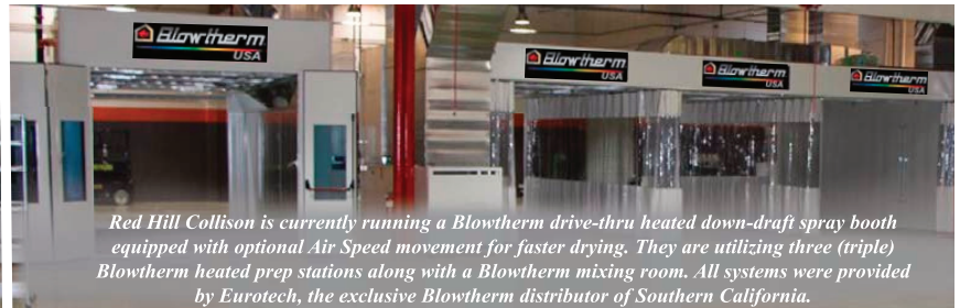
Red Hill Collision is located at 350 McCormick Avenue, Costa Mesa, CA. “...We plan on opening multiple locations throughout the Southern CA area ... all utilizing Blowtherm USA prep stations, spray booths and mixing rooms.” ~ Armando Nogueiras, CEO
