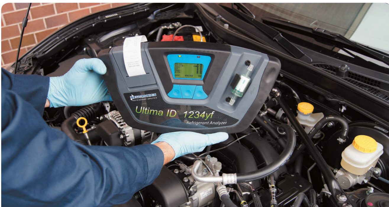
This newest model of identifier can work on R1234yf and R134a systems.
