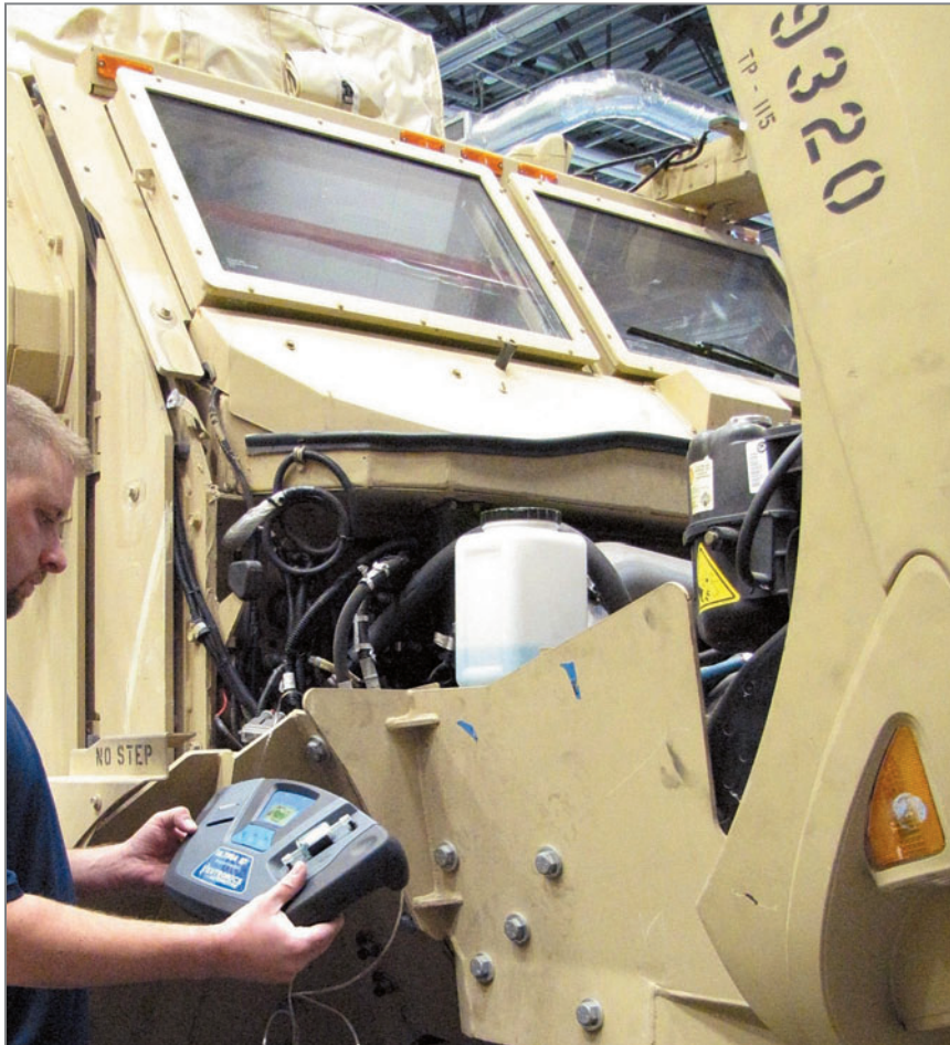
TARDEC Senior Engineer Jeffrey Marcinok uses a refrigerant identifier to field test a vehicle.
