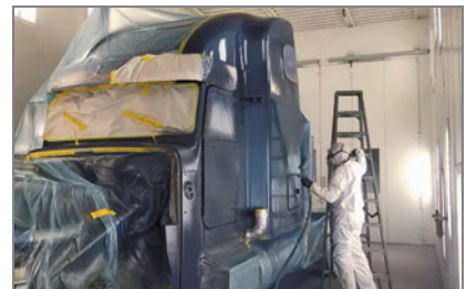
Nitrogen allows us to spray with smaller tips and at lower pressure, which keeps overspray down allowing our booth to stay cleaner.
