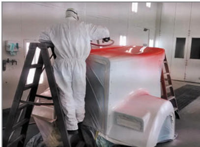
Spraying a high solid commercial finish on a Kenworth W900 hood using Ionized, heated nitrogen.
