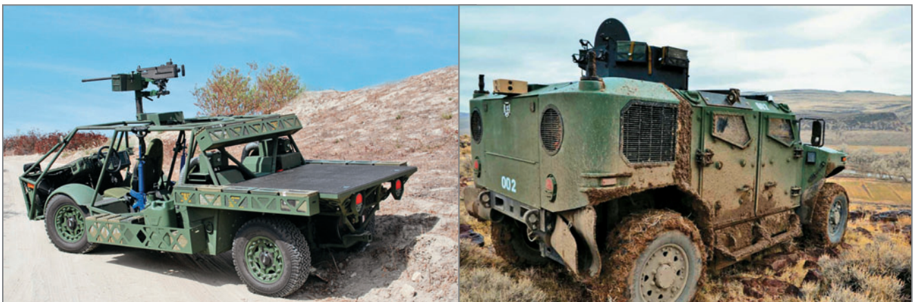
(Left) The CERV uses electric drive and can go silent (electric only) for up to 12 miles. (Right) The electric only drivetrain means better underbody protection for our soldiers from IEDs, and reduced risk by reducing the need for fuel supply convoys.
