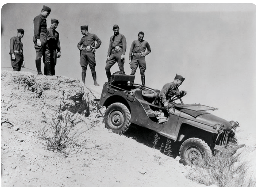
The first production version of the Bantam Jeep had fenders that were squared off. This was one of 70 initially produced for the Army.
