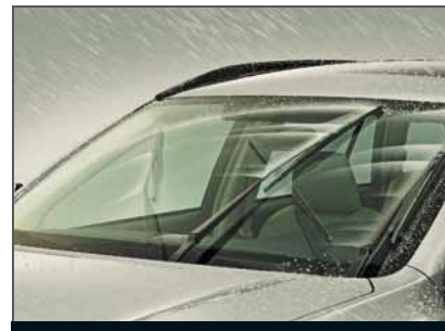
Replacement windshields with rain sensors aren't yet available from manufacturers. You'll need to recover the sensor for the old windshield and re-mount it.
