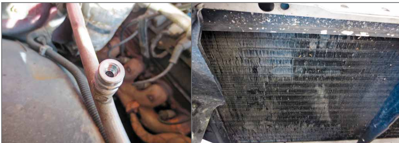
(Left) It's not unusual to have a slight leak at a charge port. That's why it has a seal with an O-ring cap. (Right) Fin damage and debris lodged in between the fins can reduce the condenser's ability to release heat.
