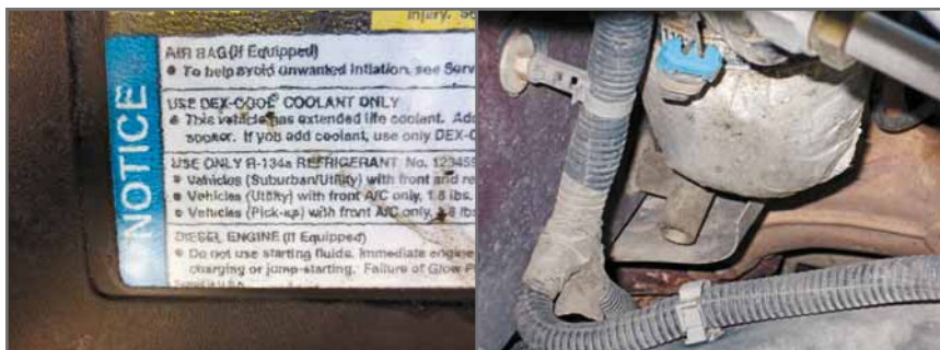
(Left) Always make sure you are charging the proper amount of refrigerant into the system. Often, TSBs are issued that alter the original charge specifications. (Right) An evaporator core leak is one of the hardest leaks to nail down. Use the drain tube or remove the blower motor resistor to gain better access to the interior of the case.
