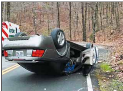
In a rollover, the windshield provides as much as 60 percent of the structural support for the vehicle roof.
