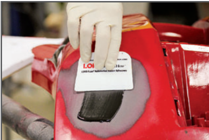
When repairing plastic automotive components apply the adhesive and spread it evenly to ensure the best adhesion.
