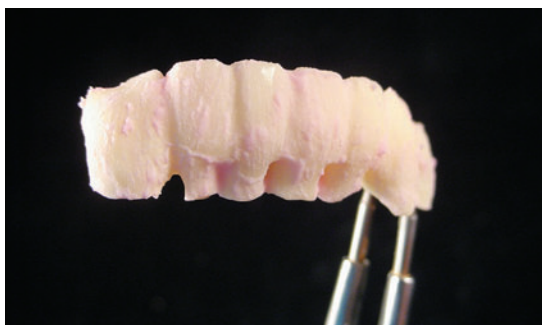
Fig. 11 The sintered bridge with support bars cut off.
