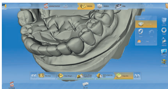
Fig. 4 Each restoration area is outlined to be copied on the biocopy model.
