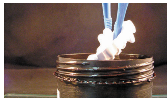
Fig. 9 Dip the framework into coloring solution.
